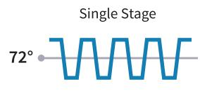
The ON/OFF operation may create abrupt temperature swings, impacting indoor comfort.
